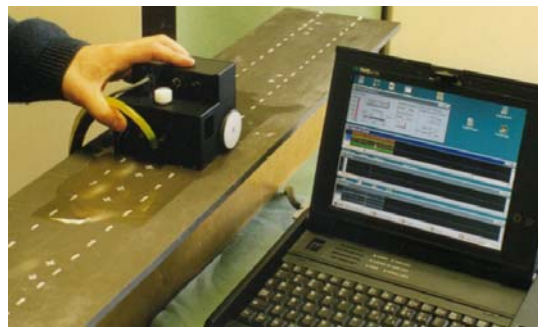
Figure 3b. C-scan imaging system on a Carbon Fibre Composite (CFC) spar.
